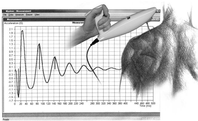
Fig. 1. The Myoton-2 device and illustration of the myometrical measuring method (design by Ivo-Ott Hirvesoo). The principle of myometry lies in giving the muscle under investigation a dosed local mechanical impulse shortly followed by a quick release, and recording the mechanical response of the muscle.
